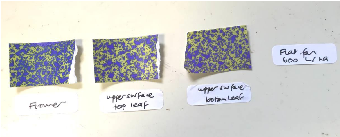
Figure 4. Spray coverage on water-sensitive paper clipped to the upper surface of top and bottom leaves and on a flower when sprayed with the flat fan nozzle 03F80 used for treatments 7 and 8.
